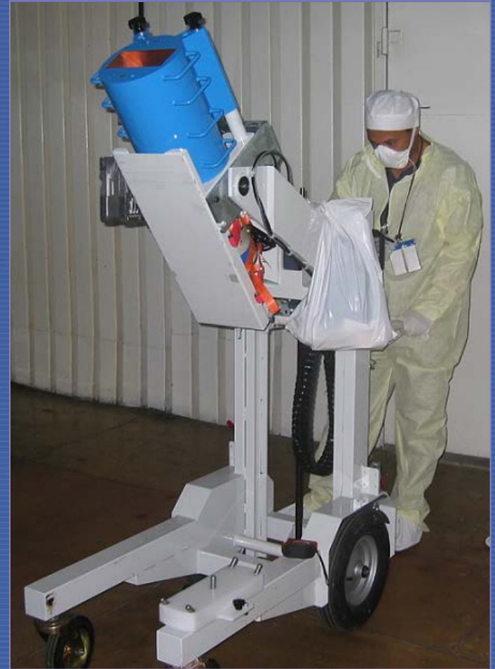
ISOCS based system for the uranium hold-up measurements (Kazakhstan)
